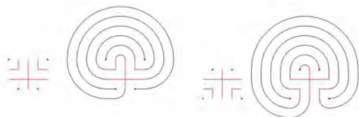
Fig. 13: Construction of the two variants of a 5-ring ancient labyrinth
