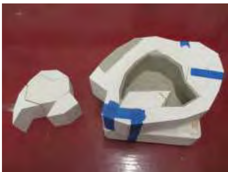
(2.5) Missing pieces (left) and liquid clay forming shell drying in their place.
