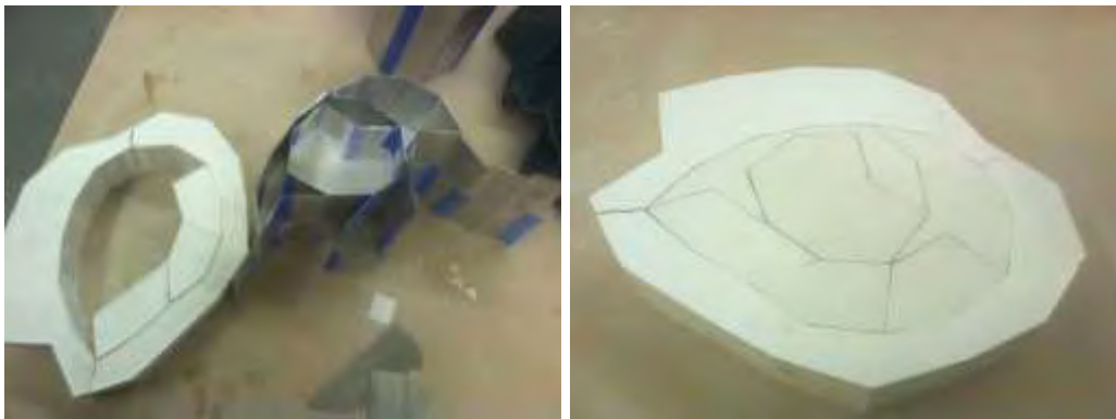
(2.3) Partially disassembled plaster pieces from metal mesh, mold configuration (foreground) fits together perfectly.
