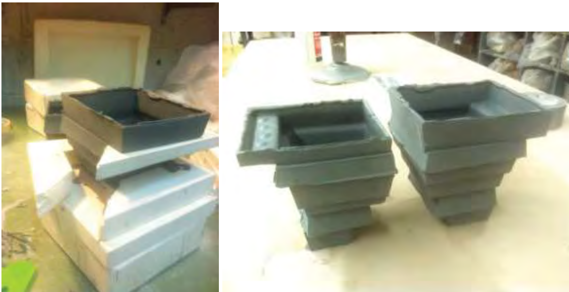
(1.7) Unmolding in progress for casting with "flip," "skip," and "slide" variations. Note split in each layer that solves draft angle problems.
