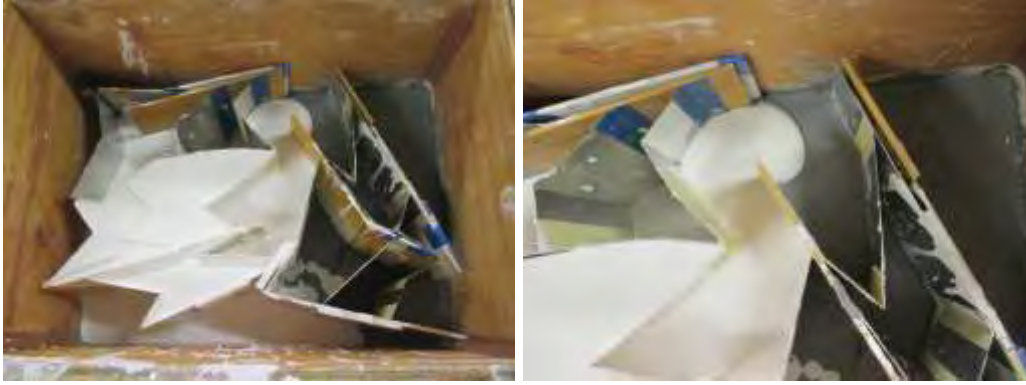
(6.7) Plaster pouring targets different areas of mesh, which fills them earlier. This means subdivisions will be at various levels.
