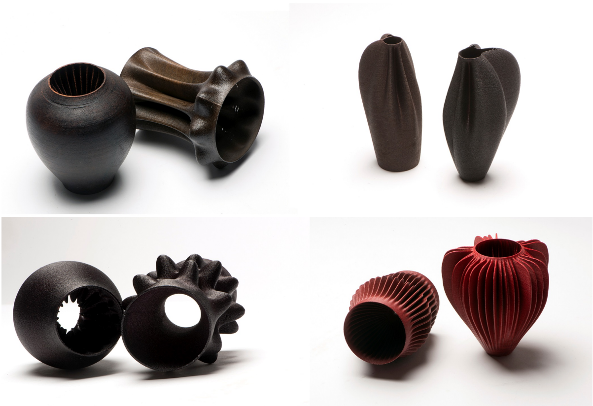
Figures 12 & 13. Post printing treatment of the artefacts by staining and surfacing.
