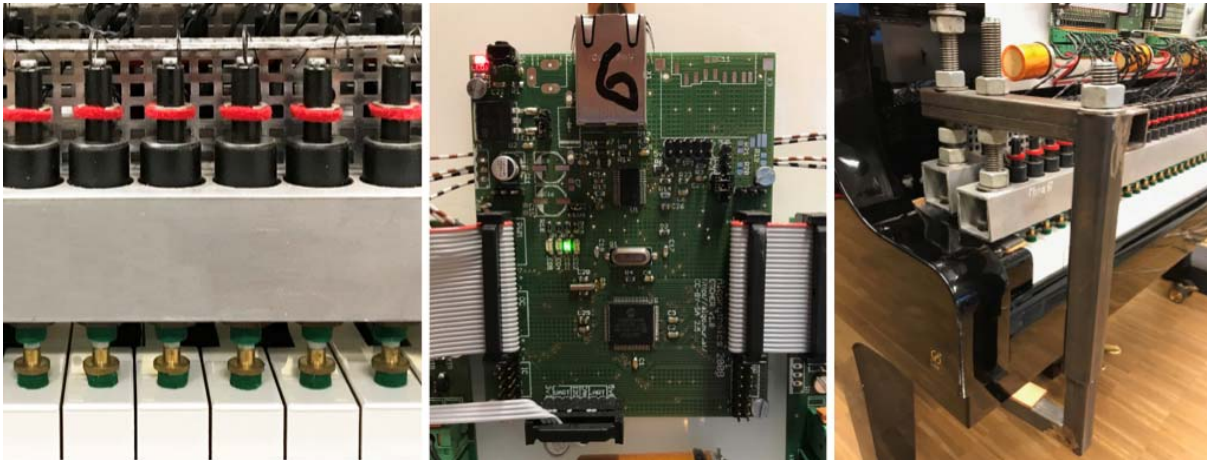
Figure 2. The solenoids, one of three microcontroller boards, one of the clamps to fix the automaton to a piano.
