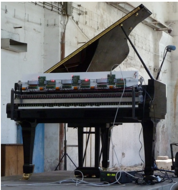
Figure 1: The piano automaton.
