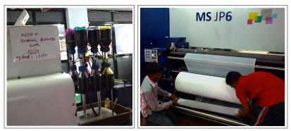
Most used fabrics for digital printing is a polyester based fabrics. The printing process should match with type of ink e.g. low energy sublimation (dye-sub), high energy sublimation (also known as disperse direct), reactive, acid and pigment. The ink chemistry should fit the requirements of the fabric (nylon, polyester, silk, cotton). On the bases of choosing fabric and ink combination, the process followed for heat-press sublimation, infra-red fixation or steaming.
