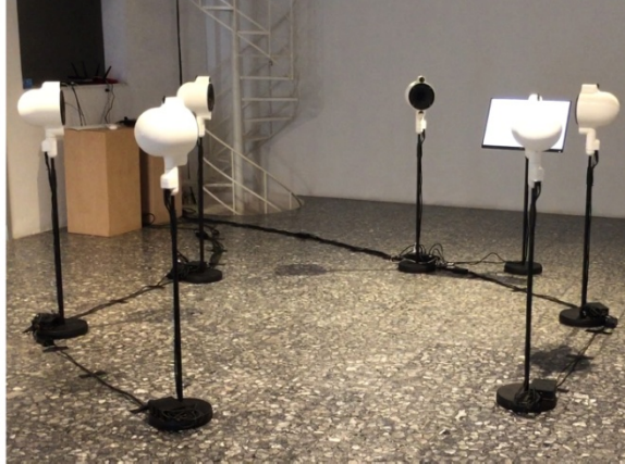
Fig 5: Watchers installation setup. The setup consists of six loudspeakers mounted on microphone stands and arranged in a ring configuration, a screen mounted on a stand, a master computer connected to an audio interface, and a Wi-Fi router.
