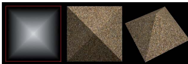
Fig. 9 Distance map of a square and its translation into a mesh
