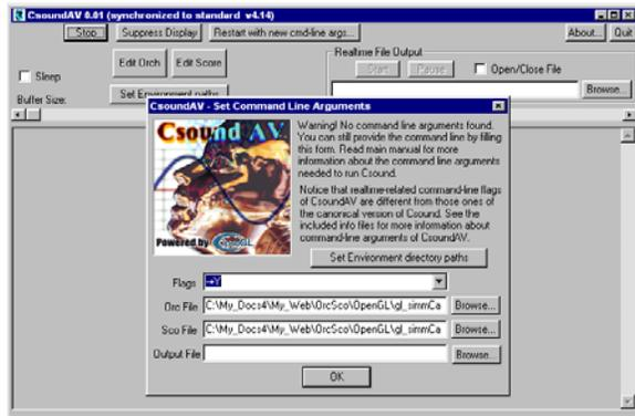
*CsoundAV* (AV standing for Audio-Video), is a major extension of DirectCsound. CsoundAV supports real-time computer graphics in both 2 and 3 dimensions, basing on OpenGL. It contains a numerous set of opcodes specific to OpenGL and graphic generation control. An additional engine (alongside normal audio engine) is provided to
