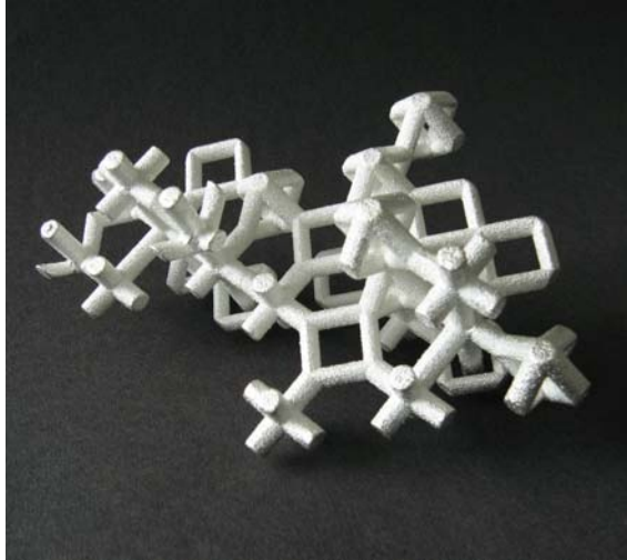
18&19 Examples of silver plated Rapid Prototyped models
