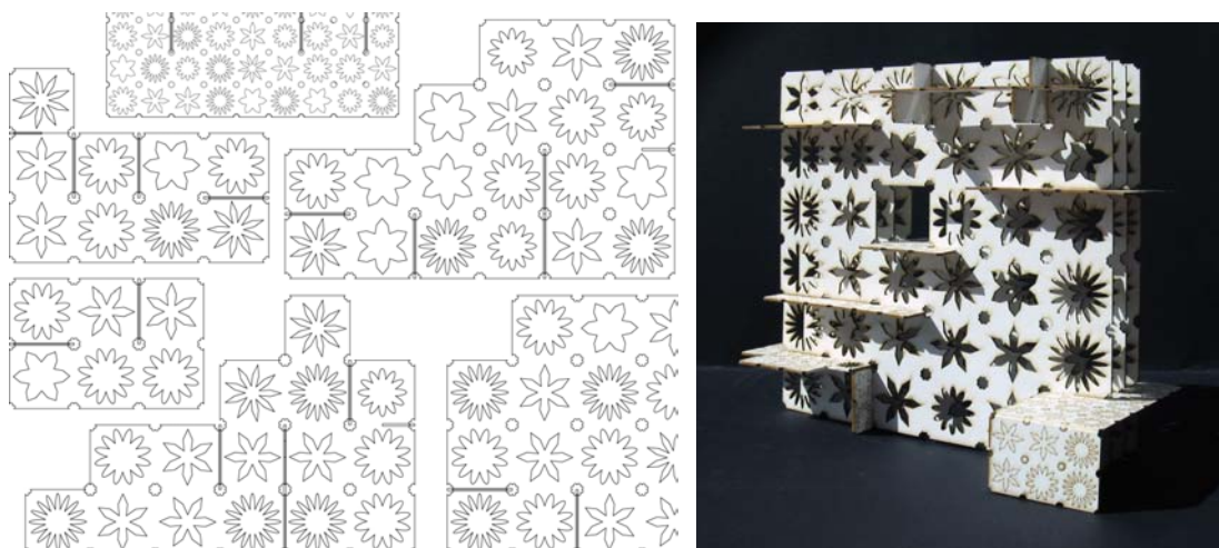
26&27 .Randomly generated patterns mapped onto flat panels for the creation of space divider, Laser cut scale model of 3mx3mx35cm space divider
