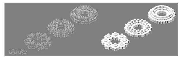
Figure 4. Initial shape and 3D representation of the polar array with 8, 16 and 32 stars.
