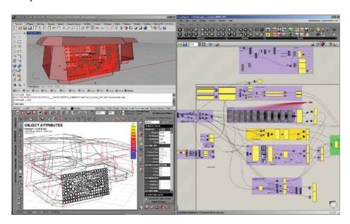
The real-time interactive model needed very fast computational time to got solutions, and forced to set a lookup table with a set of optimal solutions calculated before. The set was updated constantly in the background taking into account the new conditions and any changes related to different environmental conditions.
