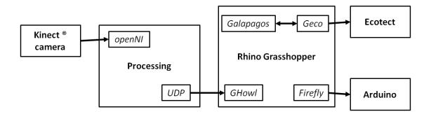
The facade collects data related to local environmental conditions through the Internet and the presence of people in the public space and spatial data with a Kinect device [6] through an infrared camera and depth sensors integrated in.
