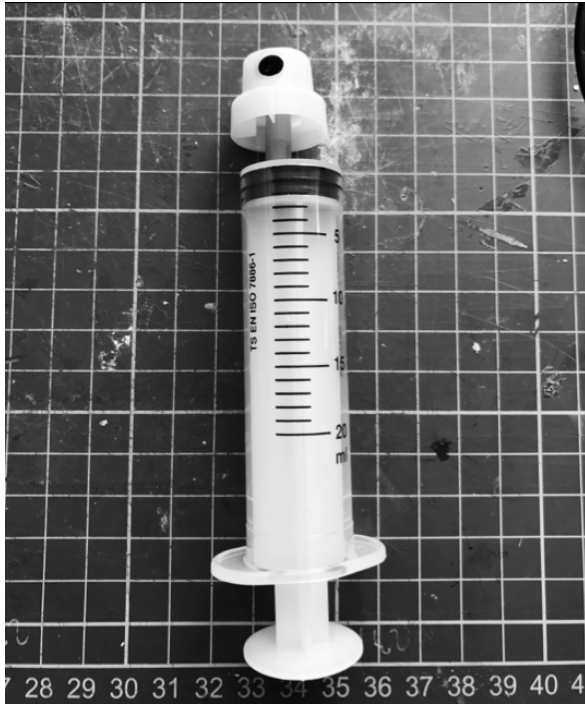
Figure.4 A syringe modified with a spray cap to achieve smooth spreaded exposure
