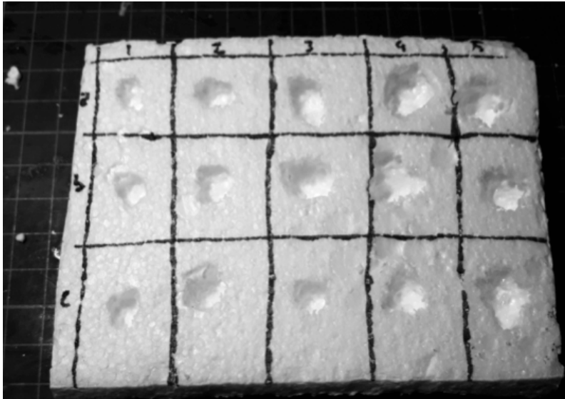
Figure.2 Identical process used in each row (a, b, c) supplies visual comparison. Each column (1, 2, 3, 4, 5) represents repeatedly increased use of solvent amount.
