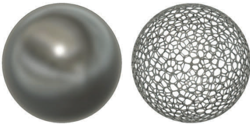
Figure 1. Comparison of a solid body and its Voronoi-based version.
