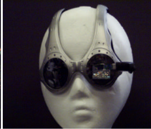
Figure 2. Fashionable wearable display projecting an image on the viewer's eye through the private-eye
