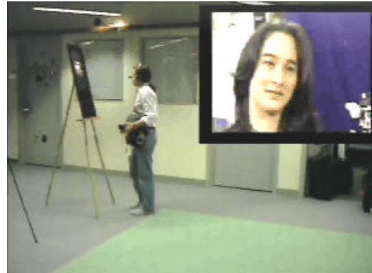
Figure 14. The Museum Wearable: an explanatory movie clip plays as the visitor approaches a printed photograph of an artwork on display
