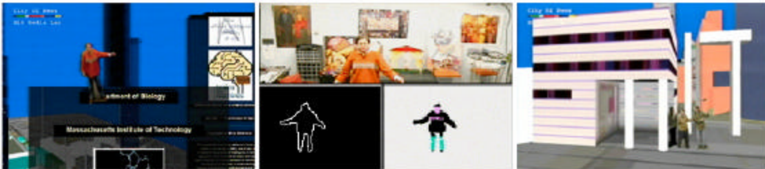
Figure 11. Virtual Studio: the user is composited in real time inside a 3-D set. In the last panel right: multiple people from remote locations are composited altogether in front of a virtual model of the MIT Media Lab.
