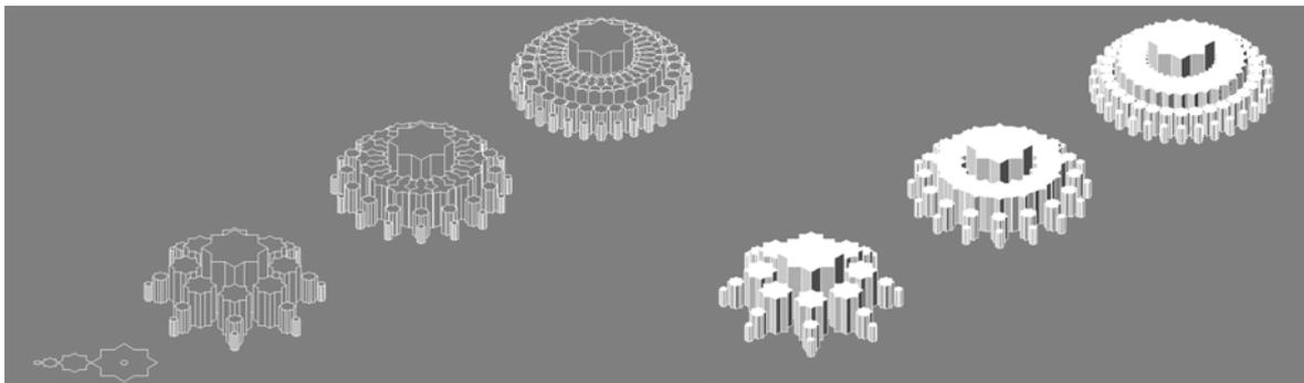
**Figure 8. Initial shape and 3D representation of the polar array with 8, 16 and 32 stars.**
