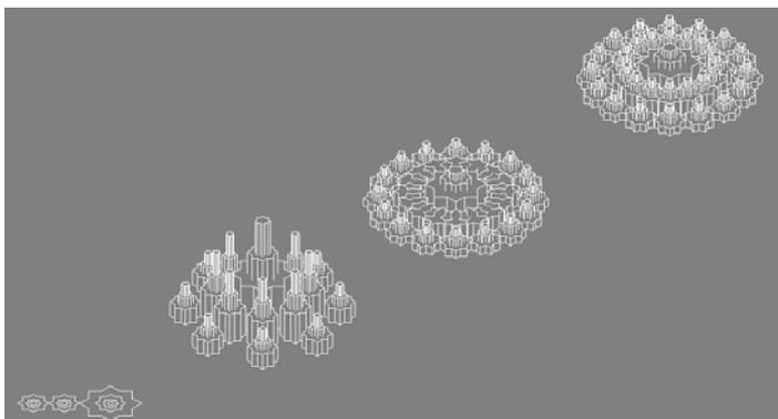
Figure 5. Initial shape and 3D representation of the polar array with 8, 16 and 32 stars.
